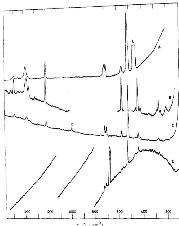
**Figure 4.** Raman spectra of solid II in  $Na_2SO_4$  (50%) for C and D. Experimental conditions [excitation wavelength (nm), laser power (mW), sensitivity, spectral slit width ( $cm^{-1}$ ), time constant (s), scan speed ( $cm^{-1}/s$ )]: A, 350.7  $Kr^+$ , 35, 1  $\mu A$ , 8.0, 4.4, 0.75; B, 488.0  $Ar^+$ , 150, 10000 counts/s, 5.0, 2, 1.0; C, 488.0  $Ar^+$ , 200, 40000 counts/s, 6.0, 2, 0.5; D, 647.1  $Kr^+$ , 100, 8000 counts/s, 5.0, 2, 1.0.
